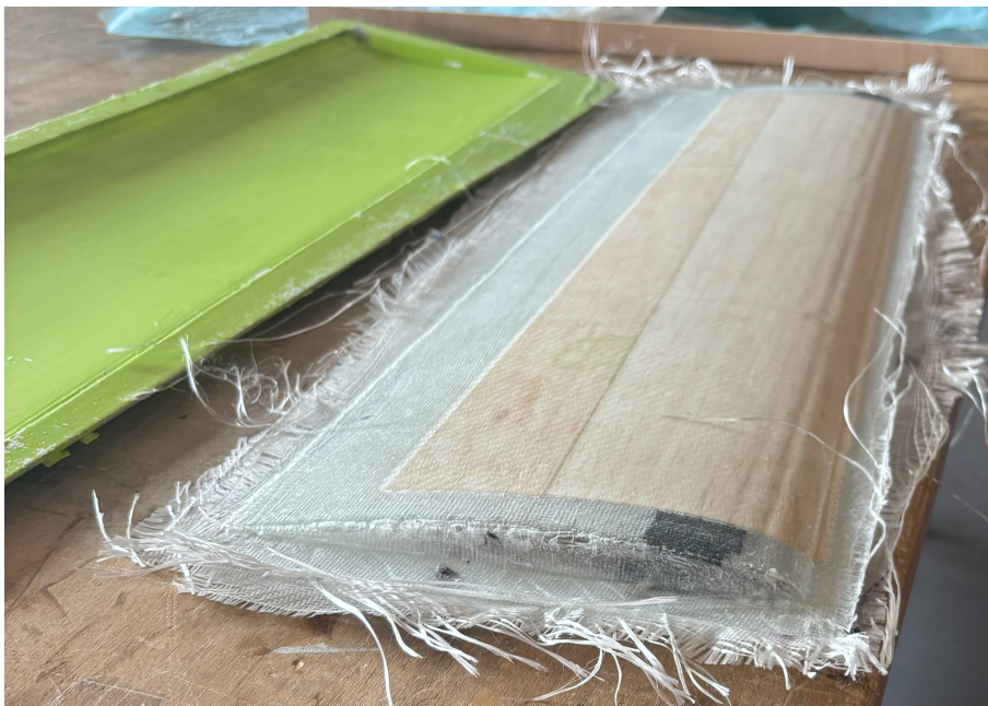
Figure 26: Post-layup of the balsa-fiberglass wing
