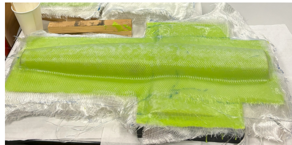
(b) Fiberglass fabric laminated over the mold and tooling coat
