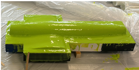
(a) Tooling coat applied to the plug and parting board
